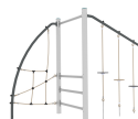
xPAL-01_ALU - NG Angular Gym N. 1 Vertical net with frame made of lamellar wood beams fixed through disappearing and passing nuts and bolts Bars realized with stainless steel tubular pegs, mounted into two lateral wooden supports Climbing cord
