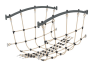
xPD-6_ALU - NG Tibetan bridge-1 NR 1 The net is made of steel strands rope, 18 mm diameter, covered with a colored nylon braid, highly resistant. The knots are covered with shell-shape protections.
