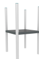
xQ-9_ALU - NG Square tower without roof h90 cm NR 1 h90 cm tower without roof made of 4 EN EV6060 anodized aluminum post with custom mold 9x9cm with rounded edges, minimum thickness 2,7mm. Central platform made of HDPE polyethylene with anti slip coating and painted and anodized steel brackets. All the fixing elements made of stainless steel
