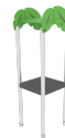
xQT4-14_L_ALU - NG Tower h140 with Roof Leaves N. 1 Composed by 4 posts having a 9 x 9 cm section by aluminium, 1 square platform placed at a height of 140 cm. Coloured polyethylene gable roof.
