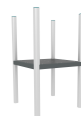
xQ-9_ALU - NG Square tower without roof h90 cm NR 1 h90 cm tower without roof made of 4 EN EV6060 anodized aluminum post with custom mold 9x9cm with rounded edges, minimum thickness 2,7mm. Central platform made of HDPE polyethylene with anti slip coating and painted and anodized steel brackets. All the fixing elements made of stainless steel
