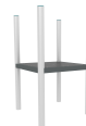
xQ-9_ALU - NG Square tower without roof h90 cm NR 1 h90 cm tower without roof made of 4 EN EV6060 anodized aluminium post with custom mold 9x9cm with rounded edges, minimum thickness 2,7mm. Central platform made of HDPE polyethylene with anti slip coating and painted and anodized steel brackets. All the fixing elements made of stainless steel
